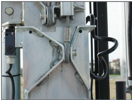
▲ Mast's external reinforcement plates on each section
