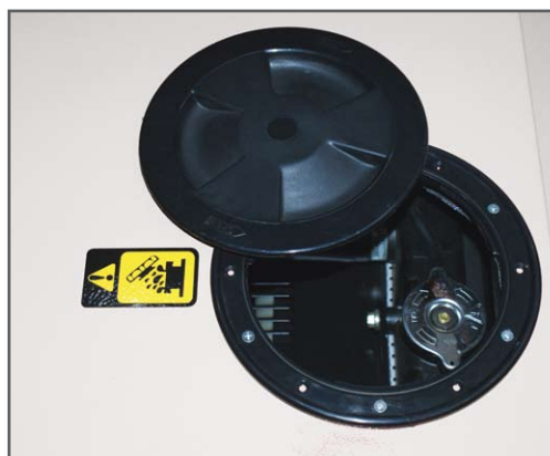
▲ Watertight "nautical" type cap to access radiator
