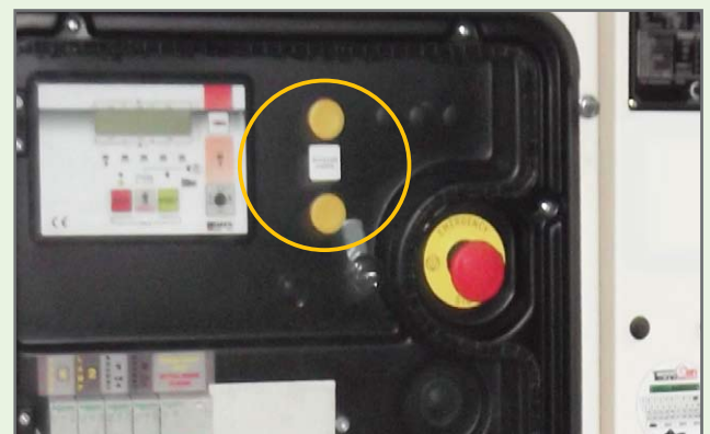
▲ Up and Down button to rise and lower the hydraulic mast
